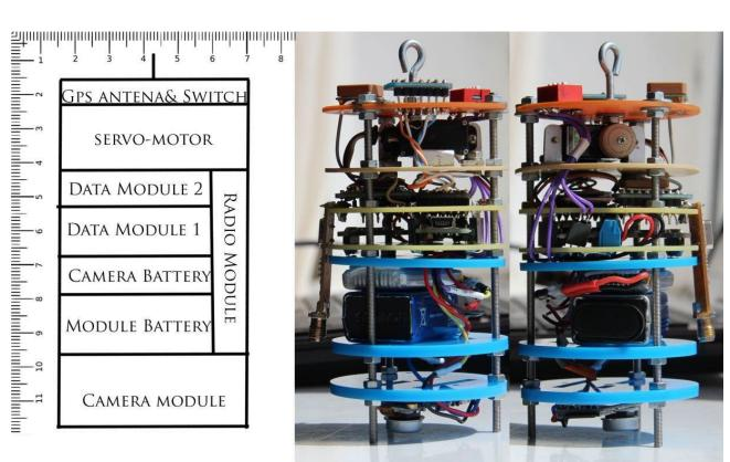
The figure above is an example of a mechanical diagram, made by a team in the 2016 European CanSat Competition. It was accompanied by a paragraph describing the purpose of each component.
